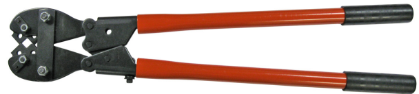
#0688T Diamond Shaped Crimp With Compound Action Exerts 5 Tons of Force Crimps 6 AWG to 4/0 AWG (250 MCM) Battery Terminals & Lugs Built In Rotating Dies for Quick Adjustment Length 25" - Weight 5.9 Lbs.
