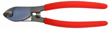
#0650PT (#0650T) Hardened Steel - Cushion Grip Handles Cuts 20 AWG Primary Wire Thru 1/0 Copper Cable (Will not cut steel)
