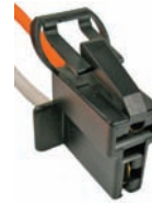
#5331PT (#5331C) Alternator Harness 2-16 ga Leads Ford 1974-77
