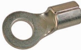
Brazed Copper Ring Terminals Electro-Tin Plated Lug Rings are Stackable Solder Or Crimp Max Temperature 295°F (146°C)
