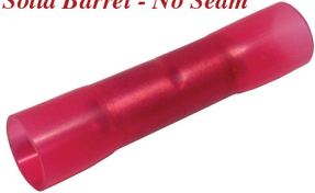
Strip Wire - Insert Into Barrel - Crimp Apply Heat Until Adhesive Flows & Tubing Shrinks
