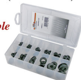
Flexible Oil Resistant Rubber Grommets Insert Into Predrilled Holes Guard Against Cut & Frayed Wires Operating Temperature -31°F to 160°F (-35°C to 71°C)
