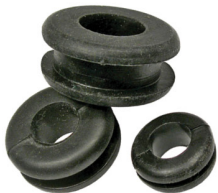
Flexible Oil Resistant Rubber Grommets Insert Into Predrilled Holes Guard Against Cut & Frayed Wires Operating Temperature -31°F to 160°F (-35°C to 71°C)
