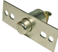
#5507PT (#5507C) Door Alarm Switch Doors - Hoods - Trunks Off When Button Pushed Spring Return to On Dual Mounting Holes 12 Volt 10 Amp
