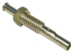
#5506PT (#5506C) Door Jamb Switch Self Grounding in Metal Panel Contact Open when Plunger Depressed & Spring Return to Ground & Closed Contact 3/8" Travel Length - 2" Overall .157" Bullet Receptacle End 12 Volt 1 Amp
