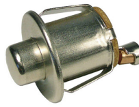
#5508PT (#5508C) Momentary Grounding Switch Push Button Momentary On Self Grounding in Metal Panel With .157" Bullet Receptacle Snaps Into 15/16" Hole 6 Volt 15 Amp 12 Volt 10A / 24 Volt 6A
