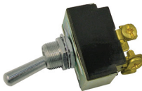
#5548PT (#5548C) On-Off Toggle DPST 3/4" Handle Length 4 Screw Terminals 12 Volt 25 Amp 125 VAC 20 Amp
