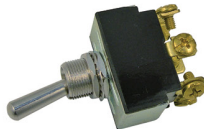
#5549PT (#5549C) On-Off-On Toggle DPDT 3/4" Handle Length 6 Screw Terminals 12 Volt 25 Amp 125 VAC 20 Amp
