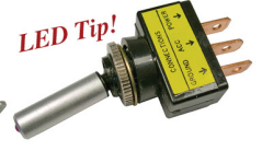
#5589PT (#5589C) Momentary On-Off- Momentary On Toggle SPDT - 3 Position Waterproof Bat Handle With Boot 3 6" 16Ga Jacketed Wire Leads 1/2" Mount Hole 12 Volt 25 Amp
