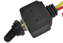
#5588PT (#5588C) On-Off Toggle SPST Waterproof Bat Handle With Boot 2 6" 16 Ga Wire Lead 1/2" Mount Hole 12 Volt 25 Amp
