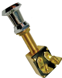
#5528PT (#5528C) Brass Marine Push-Pull On-Off SPST Switch Chrome Plated Knob 2 Brass Screw Terminals 1-1/4"x3/8" Mounting Stem 6 Volt 25 Amp 12 Volt 15 Amp
