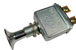
#5522PT (#5522C) On-Off Push-Pull SPST Heavy Duty Chrome Plated Metal Knob 2 Copper Terminals with 2 Brass Screws 1/2" Mount Hole 6-28 Volt 75 Amp
