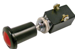
#5520PT (#5520C) On-Off Push-Pull SPST 1" Handle Pulls For On Red Illuminated 2 Screw Terminals 1/2" Mount Hole 6 Volt 25 Amp 12 Volt 15 Amp Uses Bulb #282
