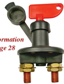
#5575PT (#5575C) Battery Cut-Off Switch Theft & Fire Protection 2 Position On-Off 12 Volt 7/8" Mount Hole Includes Removable Key Moisture Proof Cap 350 Amp DC Continual 500 Amp DC Momentary
