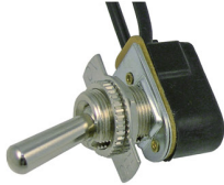
#5547PT (#5547C) On-Off Toggle SPST 3/4" Metal Bat Handle With Indicator Plate 2-16 ga Wire Leads 12 Volt 15 Amp 125 VAC 10 Amp
