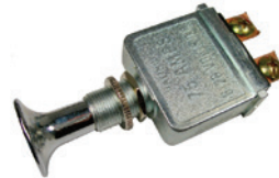
#5522PT (#5522C) On-Off Push-Pull SPST Heavy Duty Chrome Plated Metal Knob 2 Copper Terminals with 2 Brass Screws 1/2" Mount Hole 6-28 Volt 75 Amp
