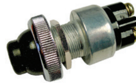
#5509PT (#5509C) Heavy Duty Push Button Momentary On Rubber Dust & Moisture Resistant Boot Nut 5/8" Mount Hole 12 Volt 60 Amp
