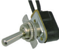
#5547PT (#5547C) On-Off Toggle SPST 3/4" Metal Bat Handle With Indicator Plate 2-16 ga Wire Leads 12 Volt 15 Amp 125 VAC 10 Amp
