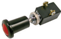
#5520PT (#5520C) On-Off Push-Pull SPST 1" Handle Pulls For On Red Illuminated 2 Screw Terminals 1/2" Mount Hole 6 Volt 25 Amp 12 Volt 15 Amp Uses Bulb #282
