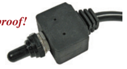
#5589PT (#5589C) Momentary On-Off- Momentary On Toggle SPDT - 3 Position Waterproof Bat Handle With Boot 3 6" 16Ga Jacketed Wire Leads 1/2" Mount Hole 12 Volt 25 Amp
