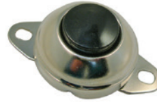
#5504PT (#5504C) Horn Button Flush Mount 2 #6 Screw Contacts Nickel Plated Housing Black Plastic Button 12 Volt 5 Amp
