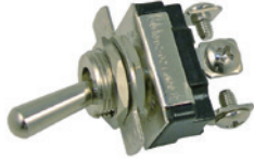
#5546PT (#5546C) On-Off-On Toggle SPDT 5/8" Metal Bat Handle With Indicator Plate 1/2" Mount Hole 12 Volt 10 Amp 3/4 HP 120-240 VAC
