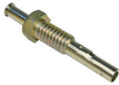
#5506PT (#5506C) Door Jamb Switch Self Grounding in Metal Panel Contact Open when Plunger Depressed & Spring Return to Ground & Closed Contact 3/8" Travel Length - 2" Overall .157" Bullet Receptacle End 12 Volt 1 Amp
