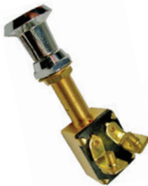
#5528PT (#5528C) Brass Marine Push-Pull On-Off SPST Switch Chrome Plated Knob 2 Brass Screw Terminals 1-1/4"x3/8" Mounting Stem 6 Volt 25 Amp 12 Volt 15 Amp
