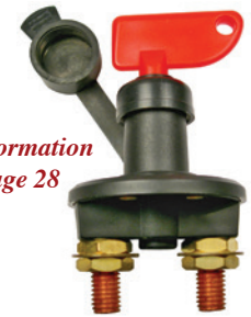
#5575PT (#5575C) Battery Cut-Off Switch Theft & Fire Protection 2 Position On-Off 12 Volt 7/8" Mount Hole Includes Removable Key Moisture Proof Cap 350 Amp DC Continual 500 Amp DC Momentary
