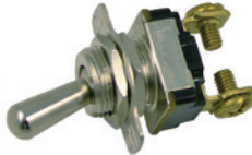
#5576PT (#5576C) On-Off Toggle SPST 1/2" Metal Bat Handle With Indicator Plate 1/2" Mount Hole 120 VAC 6 Amp 240 VAC 3 Amp
